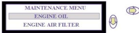
To set the interval for engine oil changes, use the down button to scroll to ENGINE OIL in the maintenance menu. to select ENGINE OIL, press the **Right button**.
