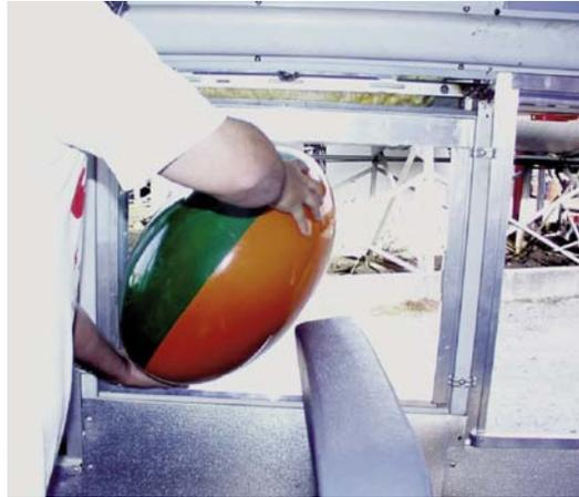
**Ellipsoid gauge passing in behind of seat back**
