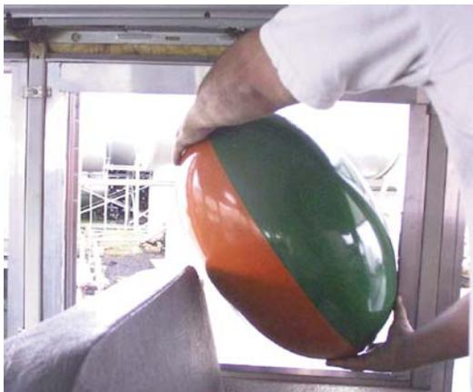
**Ellipsoid gauge passing in front of seat back**
