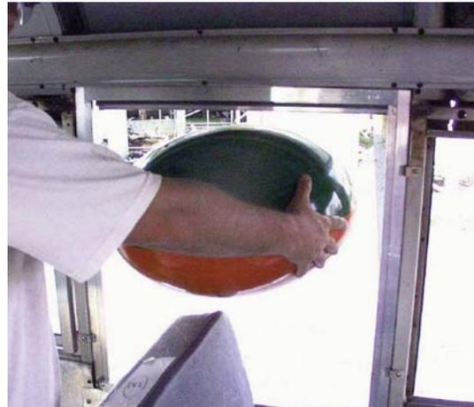
**Ellipsoid gauge passing above seat back**
